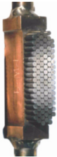
Tungsten rod component tested at 30 MW/m 2 (SNL)
